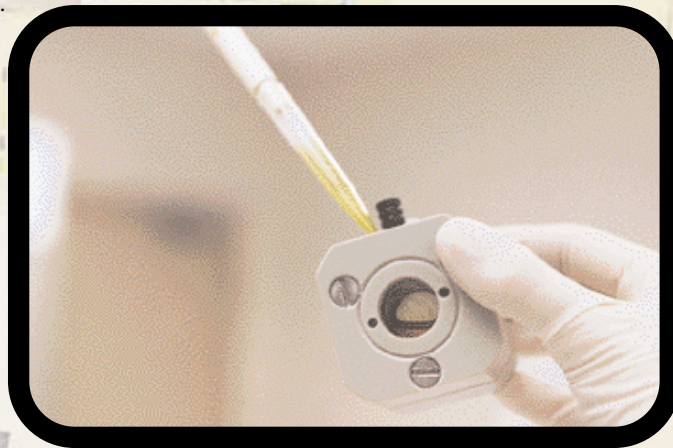
BCOP Assay – The cornea of a cow eye is held in the dosing chamber while a test material is applied. After incubation, the opacity of the cornea will be determined.
